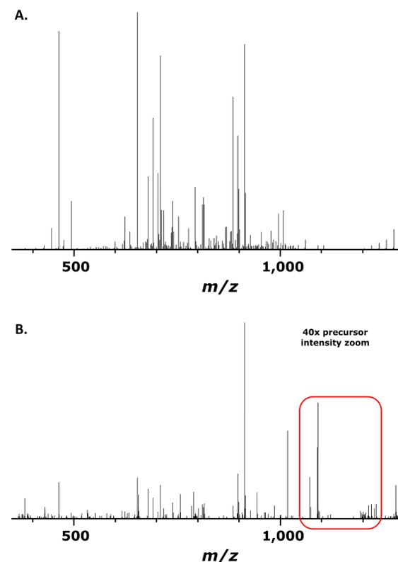
**Figure 5.** KmTx2 variant dissociation using A.) trap CID @ NCE = 50%, and B.) UVPD @ 1115 μJ. (red box) Additional ions detected after UVPD.
