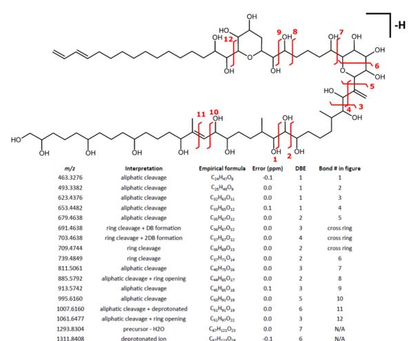
**Figure 4.** CID interpretation from FT-ICR MS/MS data for a KmTx2 variant obtained after a fish kill in China. All product ions' m/z values were determined at < 150 ppb mass accuracy.
