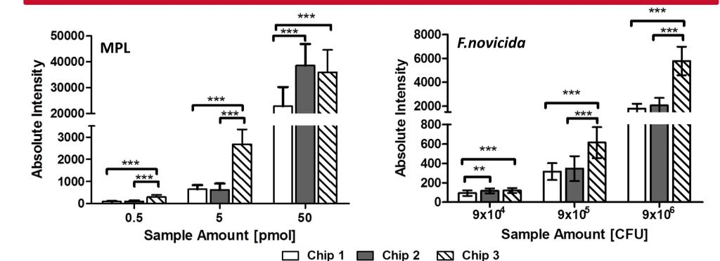
**Figure 6.** Comparison of signal intensities in SAWN-MS studies with lipid A from MPL (a) and *F. novicida* extracts (b) at three different concentrations. Shown are the signal intensities at m/z 1744 for MPL (a) and m/z 1665 for *F. novicida* (b) extracts at low, medium, and high concentrations. Data shown as mean intensities ± SD (n = 3) with one-way ANOVA, 95% confidence interval (\*\* significant at p<0.01; \*\*\*, p<0.001).
