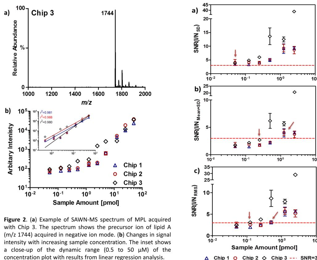
**Figure 2.** (a) Example of SAWN-MS spectrum of MPL acquired with Chip 3. The spectrum shows the precursor ion of lipid A (m/z 1744) acquired in negative ion mode. (b) Changes in signal intensity with increasing sample concentration. The inset shows a close-up of the dynamic range (0.5 to 50 μM) of the concentration plot with results from linear regression analysis.
