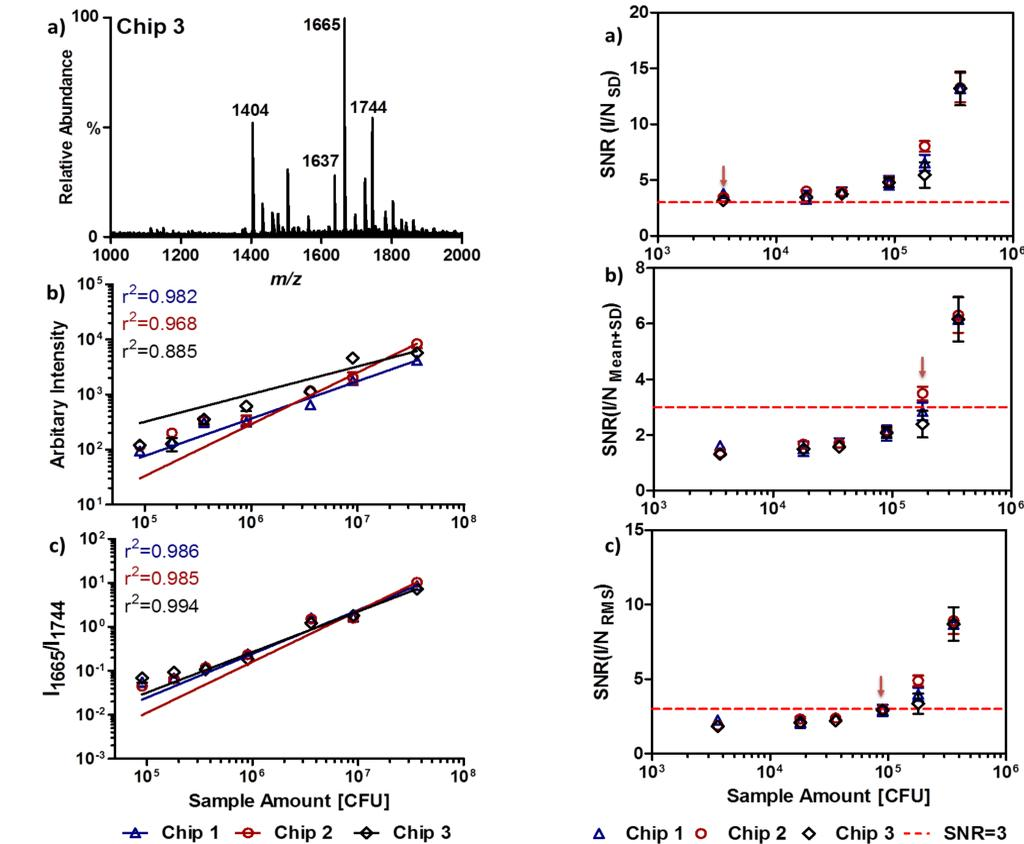
**Figure 3.** SNR of MPL in the study with three different SAWN chip designs three different methods for estimating the noise were used: (a) by SD, (b) based on the sum of average noise and SD, and (c) based on RMS of the noise. The LOD for each chip is highlighted by the red arrow in the figures above and listed in Table 1.
